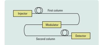
Figure 1. 2D GC utilizes a primary column (conventional separation), a flow modulator, a second column (very fast separation) and a fast detector. Compared to one-dimensional separations, 2D GC can increase peak resolution and peak capacity, resulting in a greater number of individual compounds being separated. Per unit of time, its peak-generating ability is much greater than that of a singlecolumn separation.
