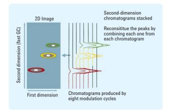
Figure 14. To visualize data in two dimensions, the modulated chromatograms are assembled as shown here
