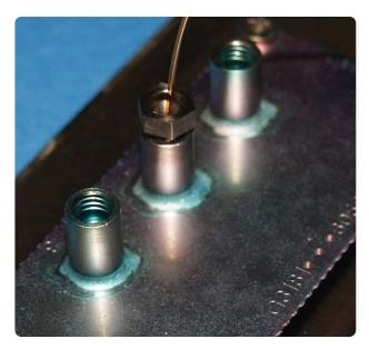
Figure 7. Close-up view of a connection to a capillary-flow device
