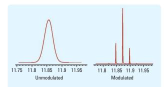
Figure 10. Unmodulated and modulated n-butylbenzene peak from a hydrocarbon test sample used to check modulator performance and timing
