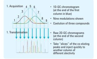
Figure 13. After GCxGC modulation, the red peak elutes last, the green peak elutes first and all three are completely separated.
