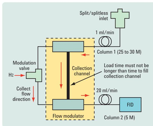
Figure 8. Flow rates and flow directions during the load or “collect” portion of the modulation cycle
