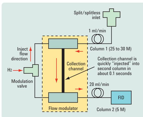
Figure 9. Flow rates and flow directions during the transfer or “inject” portion of the modulation cycle
