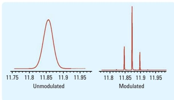
**Figure 10. Unmodulated and modulated n-butylbenzene peak from a hydrocarbon test sample used to check modulator performance and timing**
