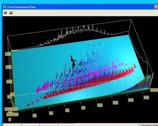
Colorized Diesel Chromatogram with Characteristic MS Grouping
